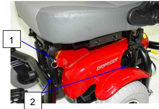
2. Adjustment pins that can be used to adjust the height of the seat to fit the user.
