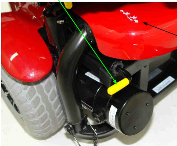
Sticker indicating position the brakes are locked or unlocked.
