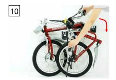
Loosen and then lower the lever to retreat the pin to release the clamping of the handle bar. Keep the crank-pedals on the level while folding the handle bar. Fold the handle bar downward toward the same side of the kickstand and beyond the level of crank-pedals.
