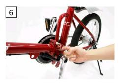
Pull out the safety pin from the locking hole.
