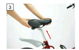
Loosen the clamp lever to remove the saddle.
