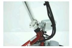
Lower the lever by fingers as shown to retreat the pin for the engagement of the handle bar. Restore the handle bar and then heighten the lever to engage pin and slot in, and then clamp the lever to secure the handle bar.
