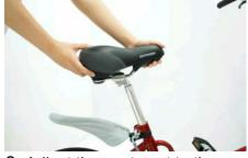
2. Adjust the seat post to the desired position.
