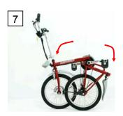
Fold the front & rear frame assembly as shown.
