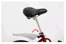
4. Tighten the clamp lever.
