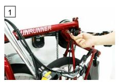
Remove the safety pin from the locking hole.
